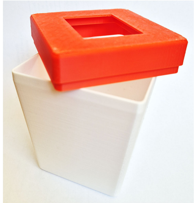
Figure 2. The plastic body of the lantern is made by 3D printing
