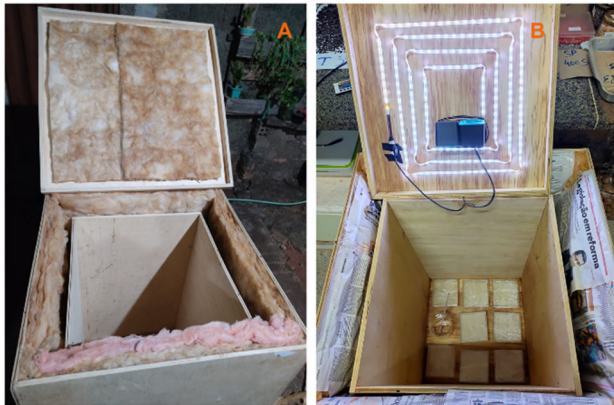
Figure 1. A) Acoustic chamber showing the outer box covered in glass wool and the inner box plus the outer cover. B) Fully assembled acoustic chamber, showing the inner lid and the presence of the LED light and speaker
