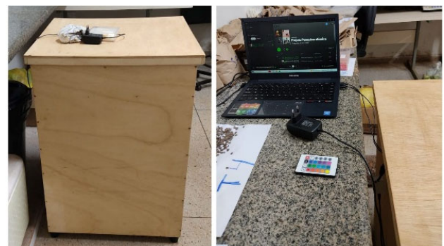
Figure 3. Complete closed acoustic chamber, identifying the use of the notebook to transmit the acoustic vibration
