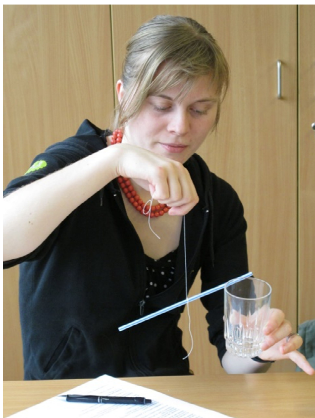
Figure 1. Electrically charged straw and glass attract each other
