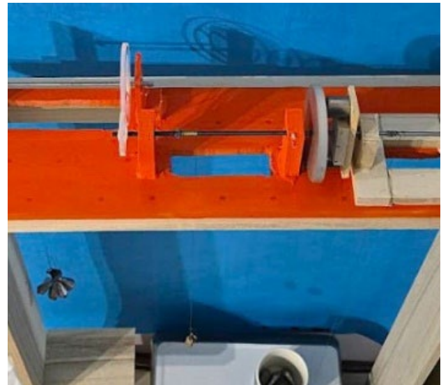
Figure 7. Torque on the large gear is applied via the weight suspended from the thread wound around its axis, while the torque on the small gear is measured using the special device.
