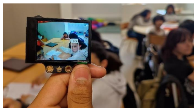
Figure 2. HuskyLens module illustrating the face-detection function
